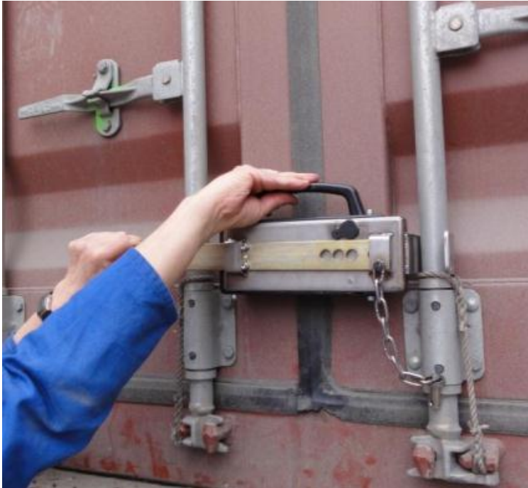
Figure 8: Installing the Container Lock on the Central Container Bars (II)
