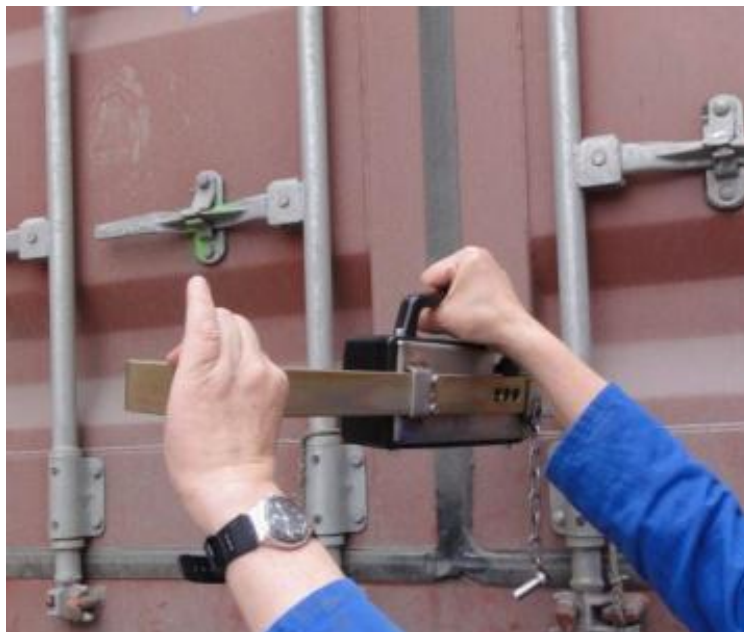
Figure 7: Installing the Container Lock on the Central Container Bars
